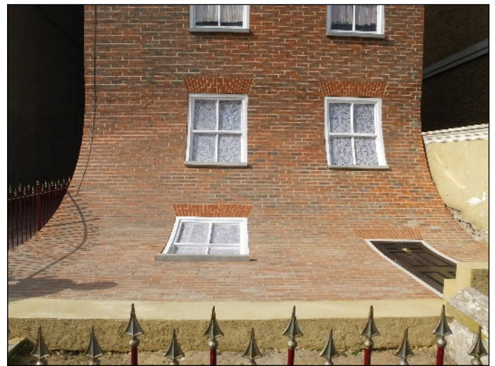
This photograph was taken at street level. To achieve the appearance of the net curtains following the curvature of the bricks, the window panes were made using two layers of curved polycarbonate with the net curtains placed in between
